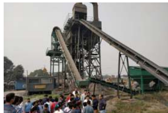
View of Hot Mix Plant, where the production capacity is 20 tonnes per hour
